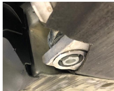
New bolt (WHT.008.757) with sleeve
